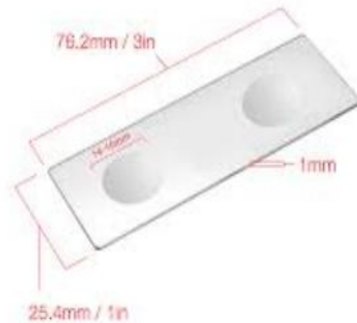
Figure 13.3: Dimensions of universal slide
