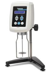
Spindle is rotated at various speeds. Then knob is also rotated in reverse order and the same numbers of readings are observed. Temperature should be very well controlled for this purpose.
