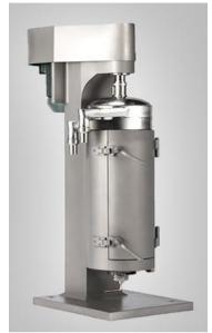
continuously from two separate holes provided on the top portion of the bowl. During clarification job, one discharge hole of the bowl is closed and continuous discharged on clarified liquid is possible. Solids accumulated inside the bowl can be removed manually after stopping machine.
