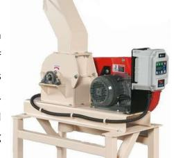
The material is crushed and pulverized (to make or crush into dust or powder) between the hammers and the casing and remains in the mill until it is fine enough to pass through a screen, which forms the bottom of the casing.
