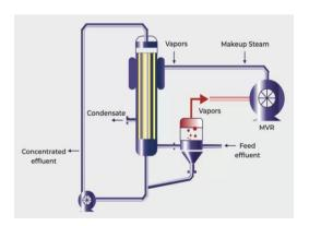
The amount of evaporation that takes place depends on the temperature difference between the steam and the solution. Problems can arise if the tubes are not well
